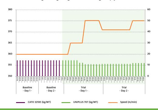
The Ingredion solution: with the use of 12kg of UNIPLUS<sup>™</sup> 707 and a corresponding 20% less wet end starch consumption, we are able to create an increase in speed by 15mpm to 375 mpm and achieve better Concora (CMT) while maintain Ring Crush (RCT), which translates into a significant five-digit cost savings per month for our customer.
